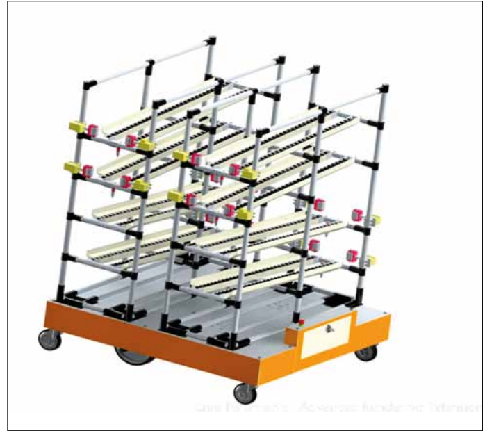
Final AGV carrying component shelves.
