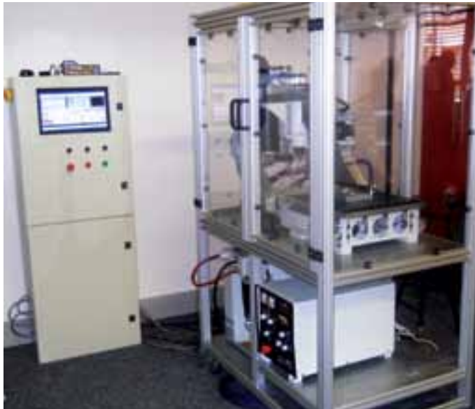
Reconfigurable machining centre developed by the GMSA Chair research group.
