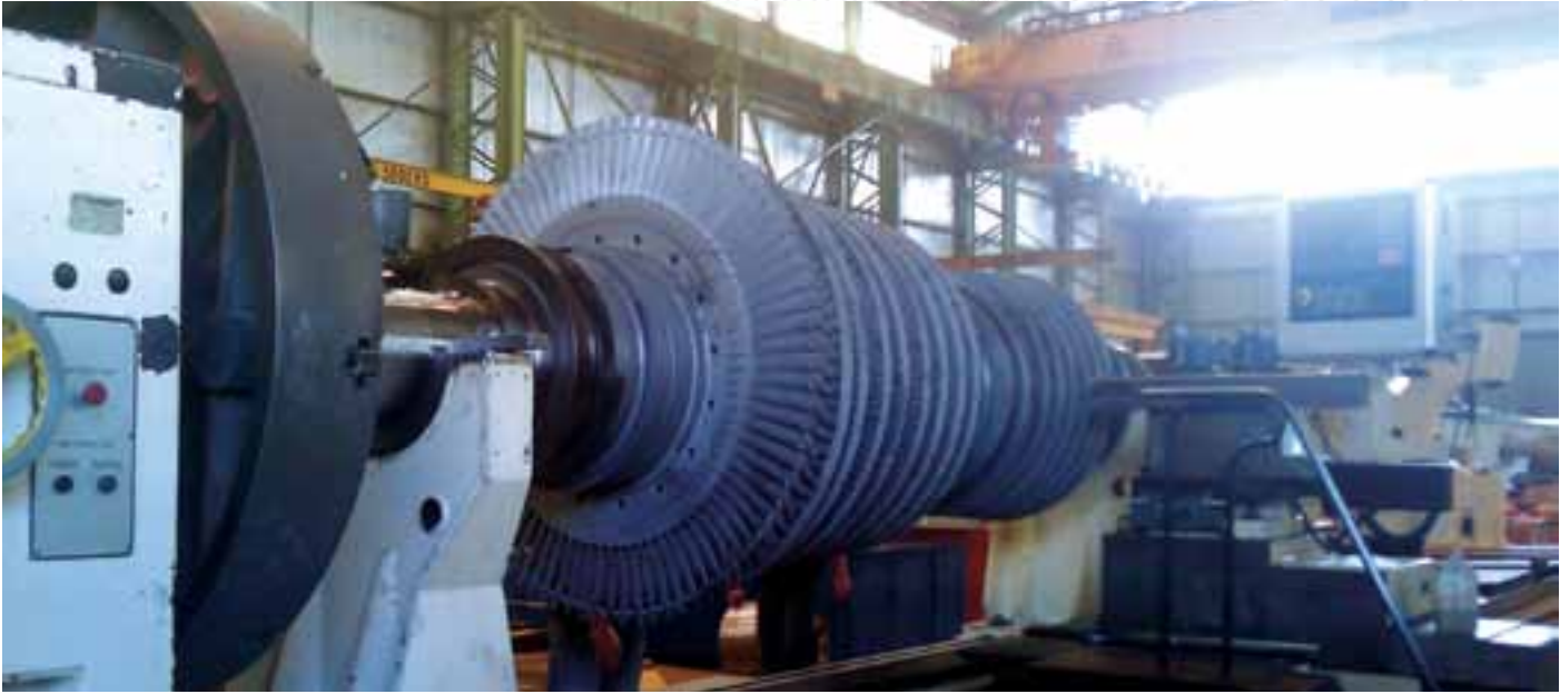
WeldCore™ process being performed on a turbine rotor disc.
