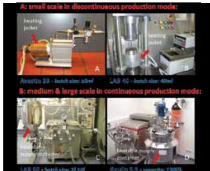
Homogenisers using high pressure to create nanoemulsions.
