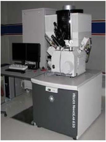
New FEI Helios FIBSEM installed in the Centre for HRTEM
