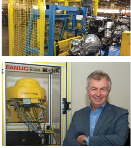
Above: New torqueing station installed in 2019 at the Isuzu engine assembly line Below: Professor Igor Gorlach
