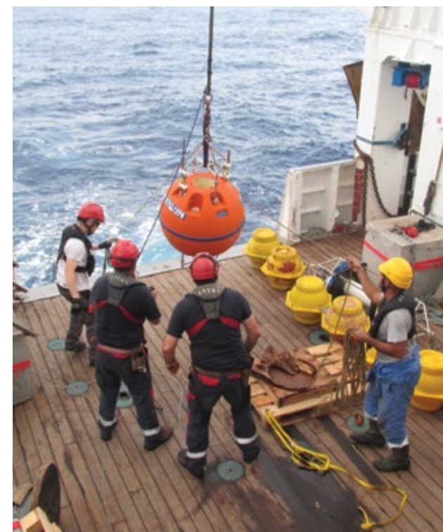
ADCP (Acoustic Doppler Current profiler) mooring being deployed at MADRidge to collect data on ocean currents, temperature and salinity. Photo courtesy Prof Mike Roberts
